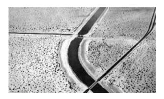
The Coachella Canal is a major branch of this system. Its turnout from the main canal is about 40 miles from Imperial Dam. The water flows by gravity about 70 miles north along the east margin of the Salton Sea to Indio, generally following the sea level contour. The canal curves west around Indio and terminates at the Lake
