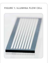
Several samples can be loaded onto the eight-lane flow cell for simultaneous analysis on the Illumina Genome Analyzer.
