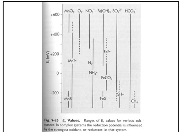
Fig. 9-26 E<sub>h</sub> Values. Ranges of E<sub>h</sub> values for various substances. In complex systems the reduction potential is influenced by the strongest oxidant, or reductant, in that system.
